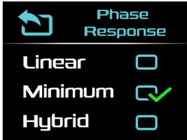
Use the three check-buttons on the PCM audio settings screen to select the Phase Response:
