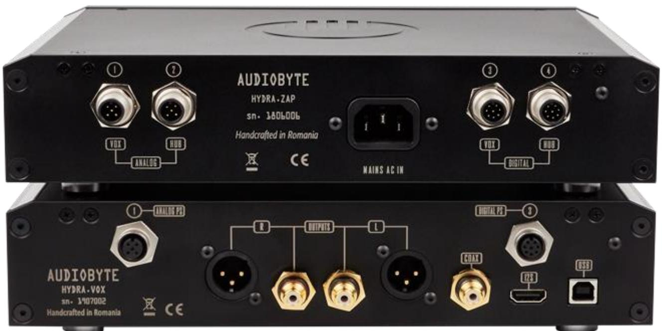
If both supply cables are correctly attached, the Audiobyte Hydra VOX is automatically powered-up when the Hydra ZAP is powered on (use Hydra ZAP touch-screen). If proper communication between the two devices has been established, a green dot will be visible near the VOX text on the Hydra ZAP main screen.
