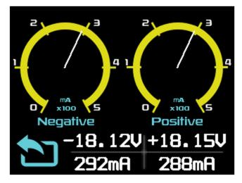
The Analog supplies monitor screen has two dials used for graphical representation of negative and positive current draw and numerical values for actual voltages and currents measured just before the output switches.
